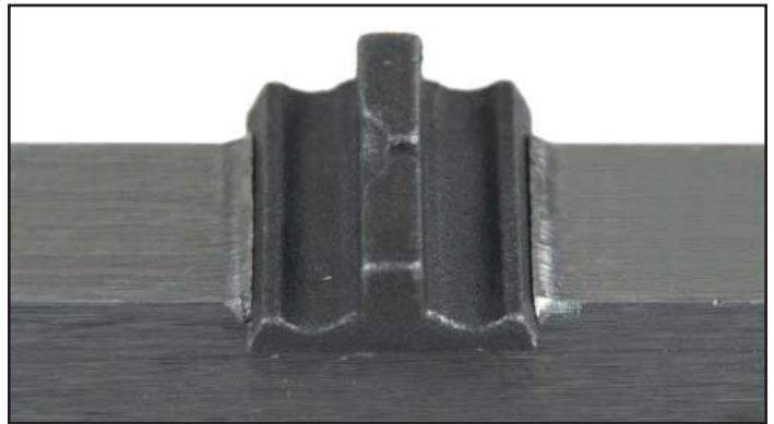
Figure 8. Installed on an octagon barrel, in a raised dovetail, the sight base is wider than the dovetail, to extend past the side edges of the dovetail slot. When zero'd, strike a center-mark across the front joint.
