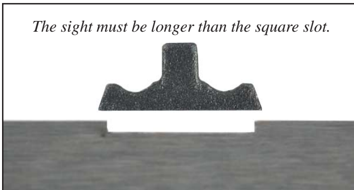
Figure 1. Cut a narrow slot for the sight or barrel lug.
