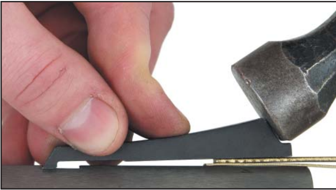
Figure 5. Place the chisel edge at a corner of the undersize slot. Hold one hand on the chisel arch, to brace it. Strike the angled flat at the rear of the chisel. Several light blows will lift an edge more easily than a single heavy blow. Rice, Colerain, Getz, Goodoien and other barrels made of 12L14 steel work easily. Green Mountain barrels are slightly harder 1137 steel. Douglas, or Spanish, Italian or other imported barrels are often drawn steel, work hardened, very difficult to form, not recommended for use with this tool.
